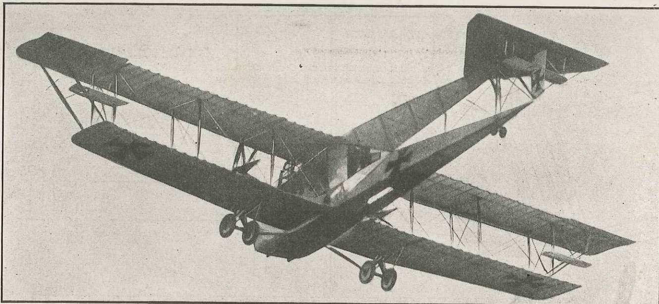
A Siemens Steffin R-1 giant bomber. Note the queer fuselage that allows firing to the rear
